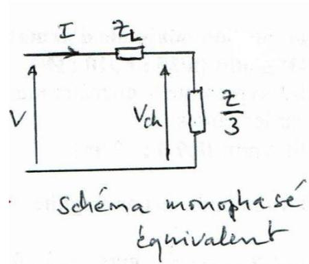
$$\bar{S} = 3\bar{V}\bar{I}^* = 3 \times 231 \times (30,16 \angle -54,03^\circ)^* = 20900 \angle 54,03^\circ = 12276 + j16915 \text{ VA}$$
