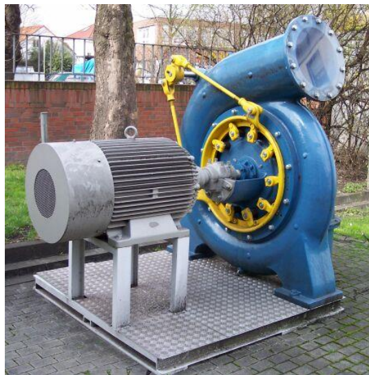
Fig.II.6. Francis-type turbine with its generator for a small hydropower plant.
