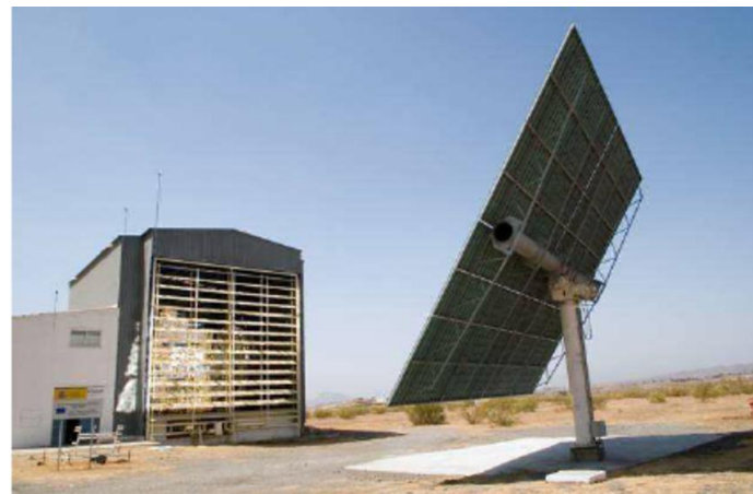
Fig.II.14. Parabolic reflector (heliostat pointed at a parabolic concentrator).
