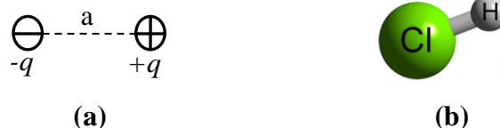
Fig.I.13. (a). Diagram of an electric dipole in its simplest form. (b) HCl electric dipole « Hydrogen Chloride ».
